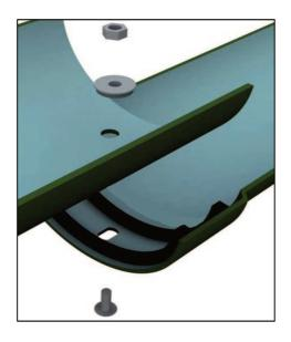
Successful jointing is achieved by applying two separate beads of Arbo 1096 gutter sealant to the inside of the gutter socket and then by using the nut/bolt/washer firmly tighten the two joints together.
