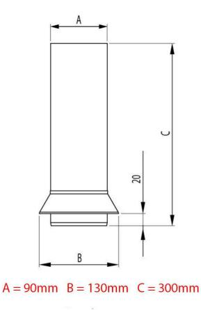
87mm Galvanised downpipe drain connector
