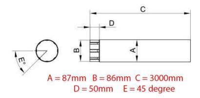
87mm Plain Galvanised Steel Downpipe Pipe for taking water flow from gutter to drainage
