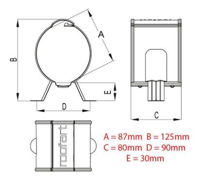
87mm Galvanised Pipe Holder designed to offer a good downpipe installation on the front part of the building.
