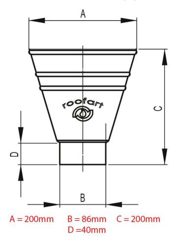
87mm Galvanised Rainwater Hopper Head
