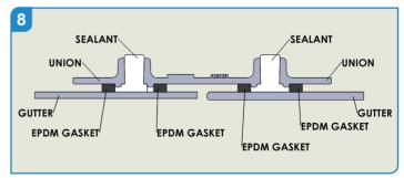
Ensure you apply the sealant gently to ensure the void is fully filled.
