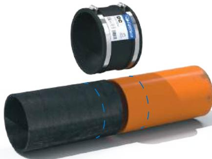
**1.** Mark both pipes, from the end to be connected, half the width of the coupling, less the required joint gap, which is usually 10mm.
